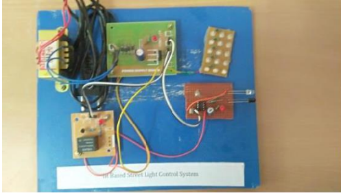
IR based street control system
