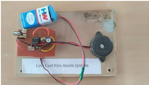
Low cost fire alarm system
